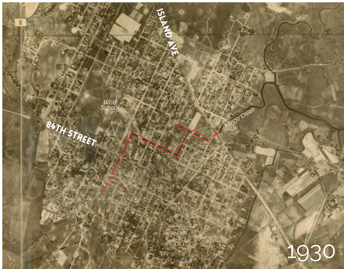
Aerial survey of Lower Eastwick in 1930, the historic drainage open channel that drained to Mingo Creek outlined in red.
