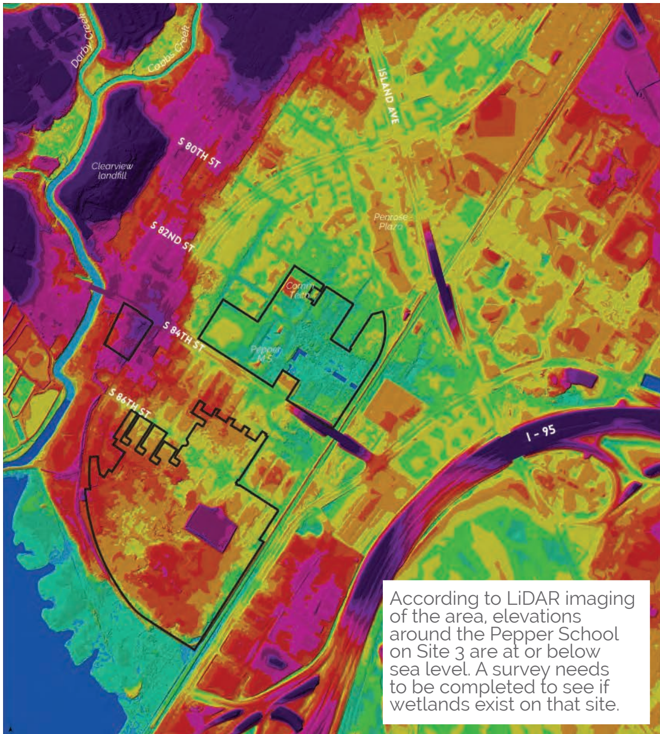
FIGURE 15: Elevation Model of Lower Eastwick.
