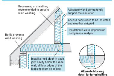
FIGURE 7.17 1<sup>1</sup>/2-story knee wall inside the air barrier
