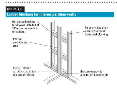
Conventional box channels for partition walls are difficult to insulate. Ladder blocking (or vertical backing, Figure 7.7) use less wood, are easier to insulate, and are easier for electricians as well. See Figure 11.3 for air sealing details.
