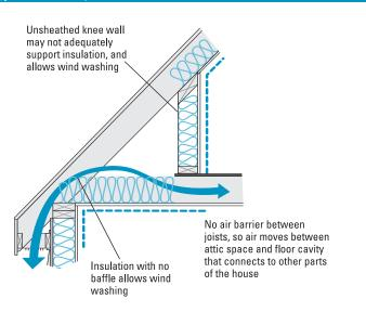
Typical knee wall details that are found in cape style homes, bonus rooms over garages, and the like are one of the largest and most common air leakage problems. This figure shows the air movement that allows outdoor air into all the joist bays, between floors. This problem can be eliminated by careful blocking of the floor framing under the knee wall, or by insulating the rafters and providing an air barrier, as shown in Figures 7.16-7.17.
