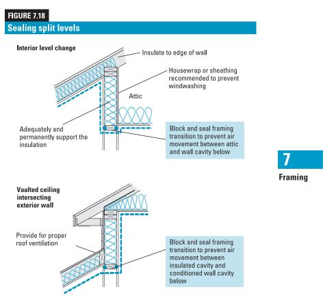
The lack of draftstop blocking in typical split-level details is another large leak. Be especially careful around stairways framed near these areas in "Tri-level" homes.
