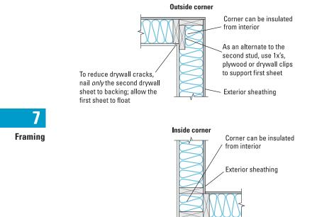
Conventionally framed corners are difficult to insulate and use more wood than insulated three-stud corners. For more savings and reduced drywall cracking, use clips for drywall backing at outside corners instead of the third stud.
