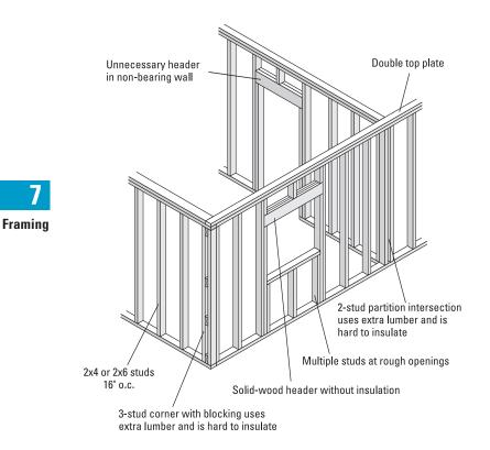
Standard framing techniques use unnecessary wood and leave less room for insulation. Advanced framing techniques are tested and proven by the National Association of Home Builders, and meet structural codes. For more detail on advanced framing (sometimes called "Optimum Value Engineering") see *Cost Effective Home Building: A Design and Construction Handbook* by NAHB (contact information in Appendix B).
