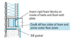
Sealing the band joist is easiest to do during framing, but if it is missed at that time, this technique works well also.
