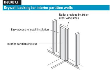
Vertical nailing stock can also be replaced by drywall clips to support drywall.
