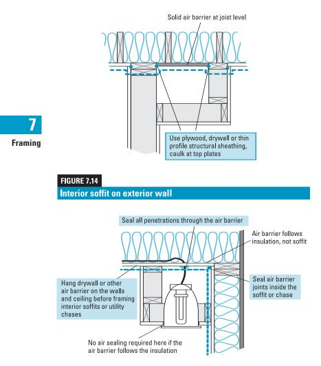
Dropped soffits are commonly built with direct air paths from inside interior walls into attics. When recessed lights are installed, heat from the lights drives air leakage even faster. Installing air barriers before framing the soffit requires coordination of framing crews and materials.
